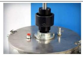
Fig. 3.Gas seal cover details.
