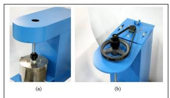
Fig. 2. Mill assembly - (a) metallic parts and (b) pulley assembly.
